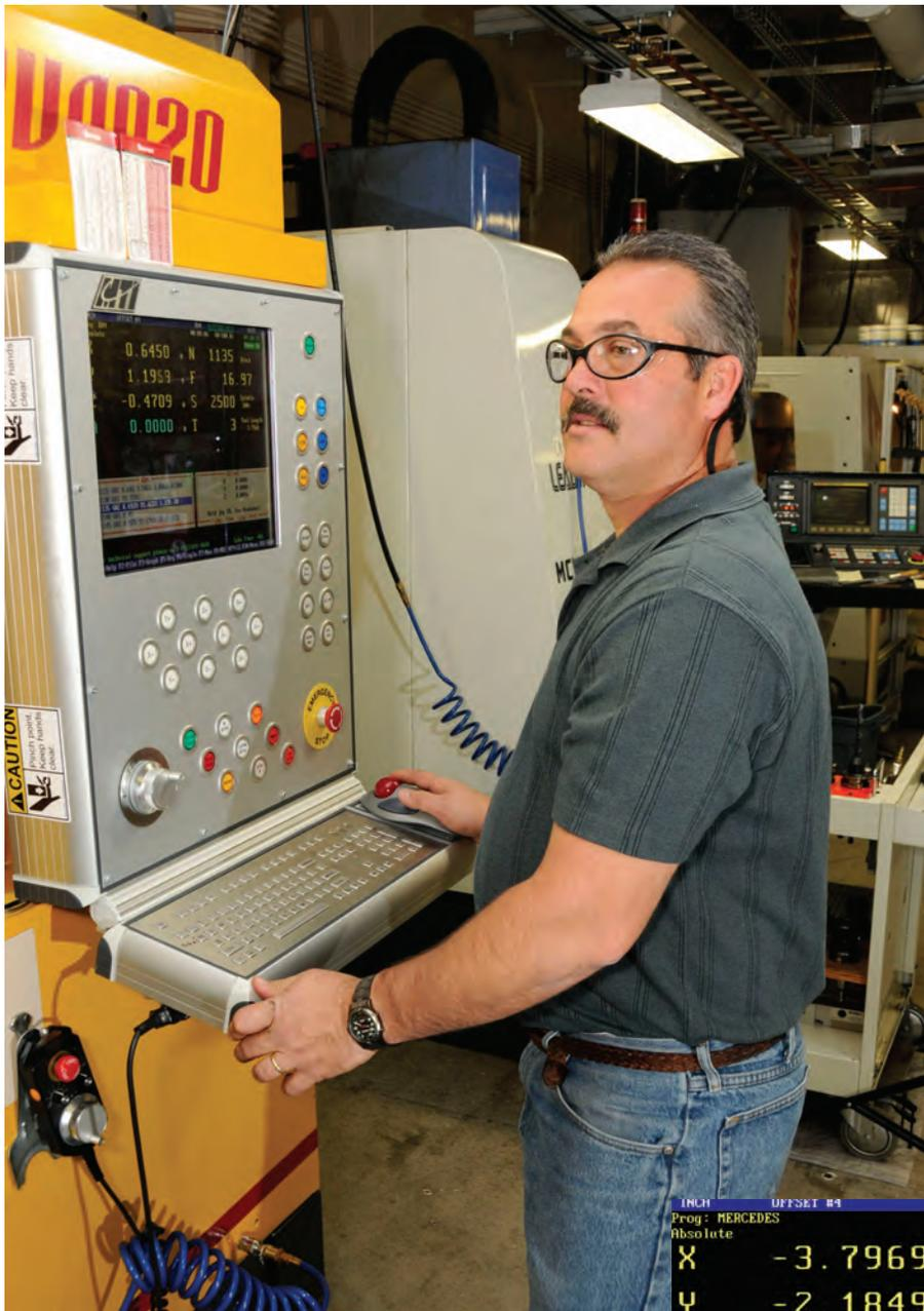
*A conventional look-ahead system relies on feedback as the machine operates; the Revolution control calculates look-ahead before the machine starts and adjusts cutter movement as the machine runs. Its data-processing capacity enables the control to monitor operations and update tool paths in real time. And 50,000 blocks/sec processing speed is the minimum achieved when interpolating eight axes; in a three- or four-axis system, the processing speed is faster.*
