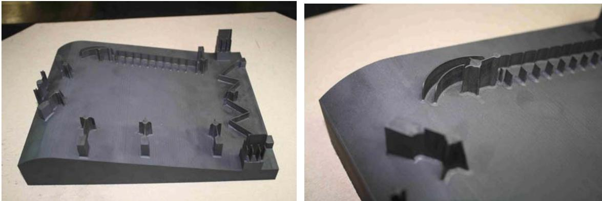
*Three close-up views of graphite electrode for a mold core slide that makes part of a between-the-seats console and CAD rendering (lower right). In the rendering, green areas represent the molding surface or area to be burned. Light blue areas indicate clearances to avoid interfere with other areas in the tool. This job is for an automotive customer.*
