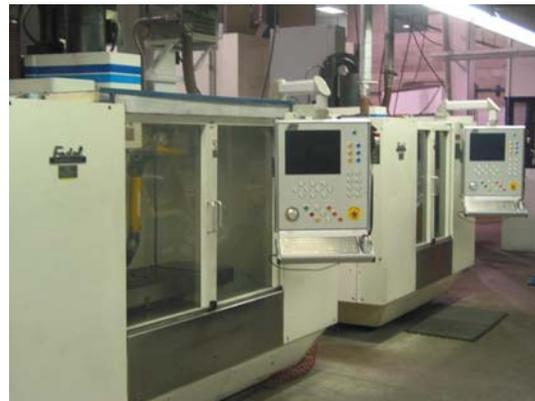
*Above left is a CAD rendering of a graphite electrode for a mold cavity that makes an automotive air-cleaner housing. Green areas represent the molding surface or area to be “burned” with EDM. Light blue areas indicate clearances to avoid interference with other areas in the tool. Above right are Michael Tool’s two Fadal 4020VMCs retrofitted with Miceli CVC controllers.*
