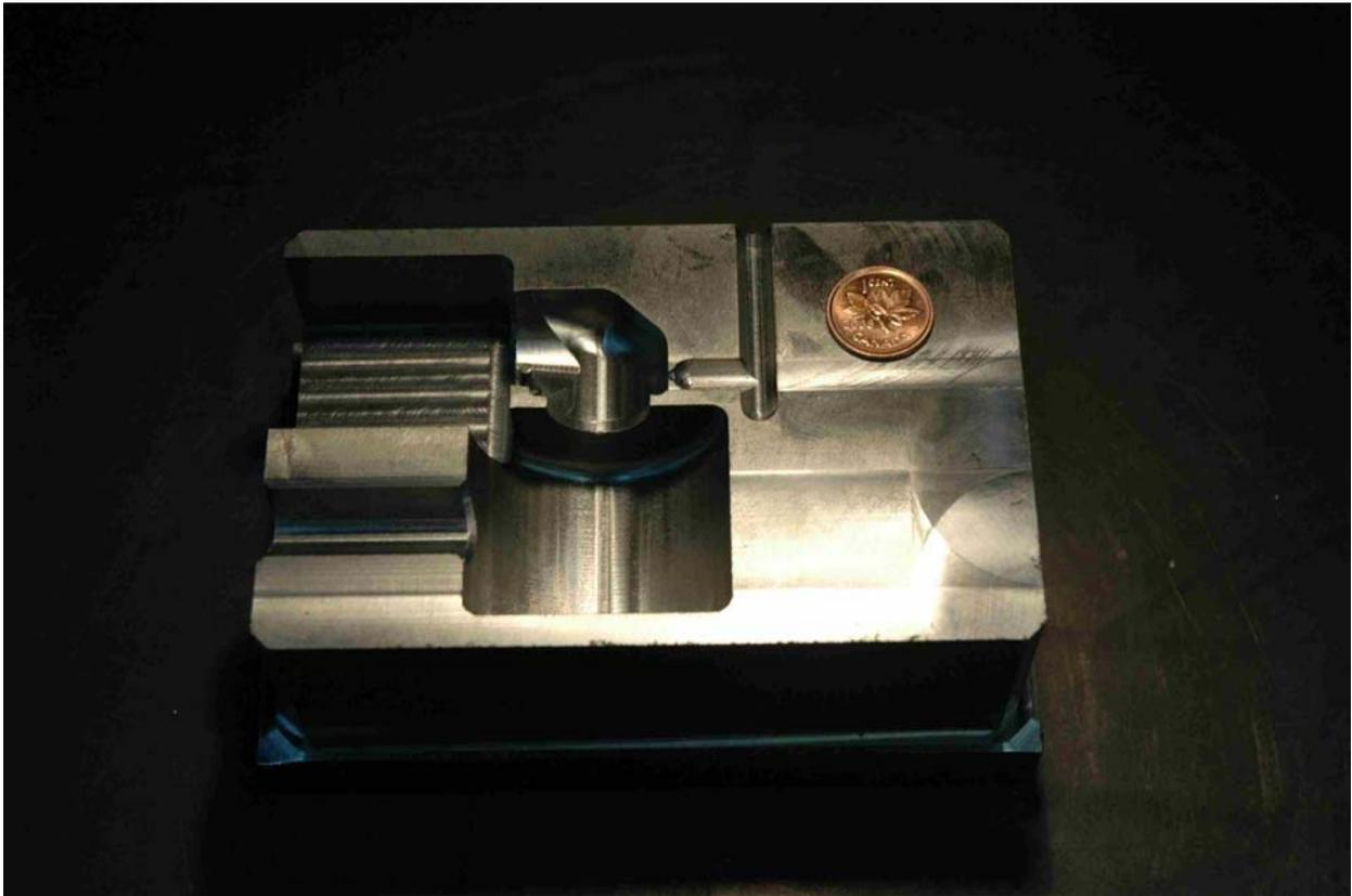
Cable-over mold tooling for injection-molding protective coverings on connections in seismic cables. Thanks to a uniquely powerful constant velocity cutting (CVC) machine tool control from MTI Fidelity Machine & Mould Solutions (Calgary, Alberta, Canada) turns these products out in large numbers.
